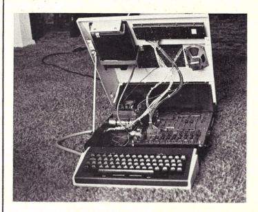
Internal view showing added wiring (note speaker for internal sound).
